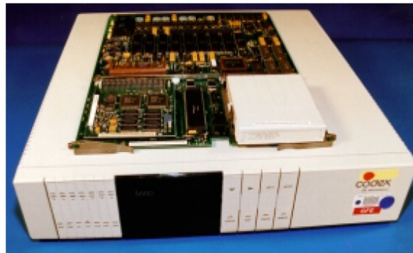
Codex 3600 Modem that Used a Higher Symbol Rate and Trellis Precoding to Attain Transmission Rates of 24000 b/s
