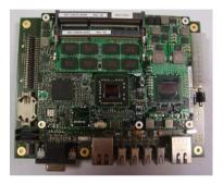
Deploying PowerPC Core IQ or Celeron M,Pentium M, Core 2 duo ,Atom or i5, I7 Gen3 up to 2.53GHZ and 16GB RAM,Dual Gigabit Ethernet port, 4 USB ports,video ,CFAST, Sata ports operating temperature 0°C to 60° C and -40°C to 85° C operating systemWindows,linux,VxWorks
