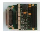
FMC Dual or Quad ARINC429 2Receive /2 Transmit channels or 4 Receive/4 transmit channels
