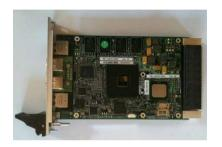
Deploying PowerPC Core IQ or Celeron M,Pentium M, Core 2 duo ,Atom or i5 I7 Gen3 up to 2.53GHZ and 16GB RAM,Quad serial ports RS232/422/485, three Gigabit Ethernet ports, 6 USB ports, 8 GPIOports, video ,CompactFlash , Sata ports operating temperature 0°C to 60° C and -40°C to 85°C operating system Windows,linux,VxWorks
