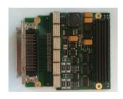
FMC Dual CAN BUS and 2Receive /2 Transmit ARINC429 channels
