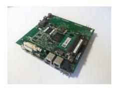
Deploying PowerPC Core IQ or Celeron M,Pentium M, Core 2 duo ,Atom or i5, I7 Gen3 up to 2.53GHZ and 16GB RAM, Dual Gigabit Ethernet port, 3 RS232/422/485, dual XMC or PMC slots,CompactFlash, 4 USB ports,video , Sata ports operating temperature 0°C to 60° C and -40°C to 85° C operating system Windows,linux,VxWorks
