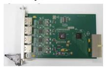
CompactPCI3U Quad Gigabit Ethernet operating temperature -40°C to 85° C operating system Windows,linux,VxWorks
