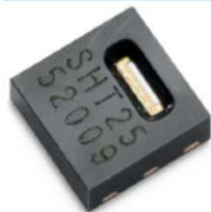
Humidity sensors from Sensirion in handsets from Fujitsu and Chinese OEMs since 2010. API available in Android
