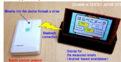
Just blowing into the device, it gives an estimate of how much fat you are burning and your hunger levels Gas sensor to monitor fat burning and hunger level (NTT docomo, March 2012)
