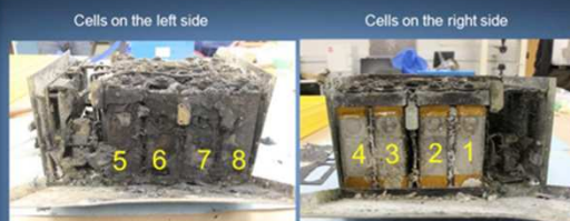
Substantial thermal damage
