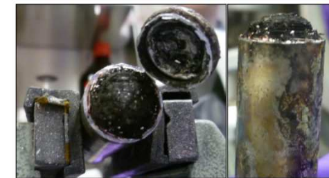
Figures 17 : DEF 1- Cell opening – positive pole
