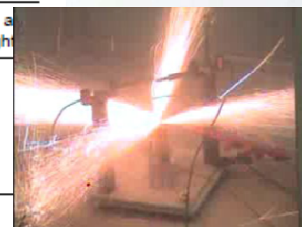
Degassing and Fire with 18650 Cells after Abuse Tests (source: es116_cunningham_2012)
