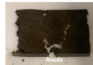
Locally Aluminum current collector has melted during the thermal runaway
