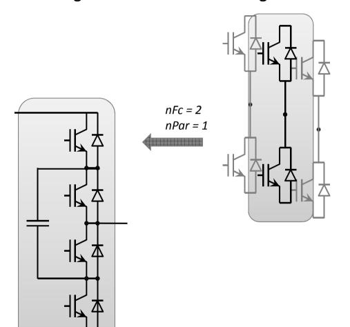
• *nStack, nFc, nPar* are parameters for the multilevel switching cell
