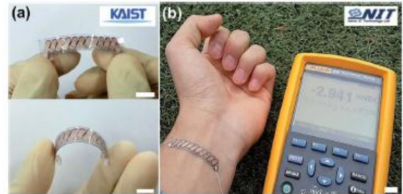
Fig. 6 Demonstration of band-type flexible TE generator for harvesting thermal energy from human skin: (a) photos of band-type flexible TE generator and (b) electricity generation measured on human skin at an air temperature of 15 °C. Scale bar, 1 cm.
